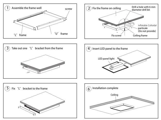
! Please make sure the frame is assembled well before fixed on ceiling.
