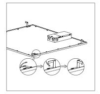
5. Insert luminaire into T-bar ceiling grid. Secure safety cable to connection hole as needed to meet local seismic requirements. Safety cable and method of attachment to the building provided by contractor according to local building codes.
