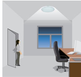
2. Any movement is detected from any direction, all lamps synchronously switch on.
