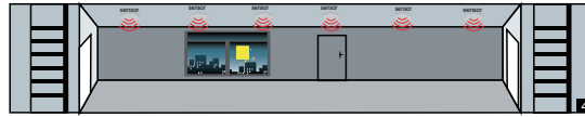
4. After stand-by period, the lamps switch off if no movement is detected in the detection zone.
