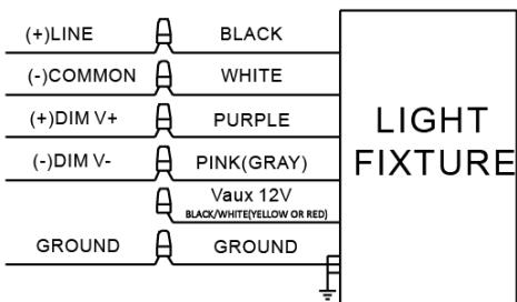
4. Connect the purple fixture lead to the (V+) DIM lead.
