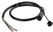
LCB-5PIN 5-pin leader cable with female plug and waterproof cap 2xAWG17+3xAWG20 20" length
